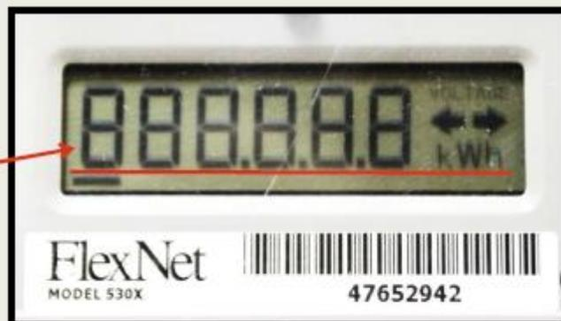
Meter will display **OPEN** only when meter has been disconnected.
